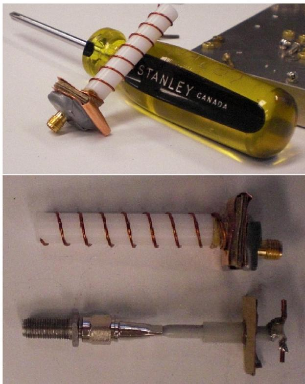
Figure 4.3: Prototype helical antenna
