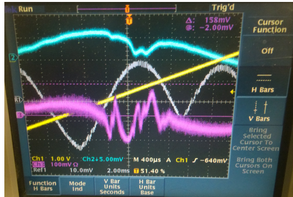
Figure 3: Saturated absorption spectroscopy based PDH signal acquired near the start of the project. Shown is the ramping signal (yellow), AOM-based reference saturated absorption spectrum (blue) and the new EOM-based PDH signal (pink). This signal is suboptimal due to low SNR (approximately 3:1), which was difficult to improve given available resources. Additionally, AM pickup effects bring into question the accuracy of the zero crossings.
