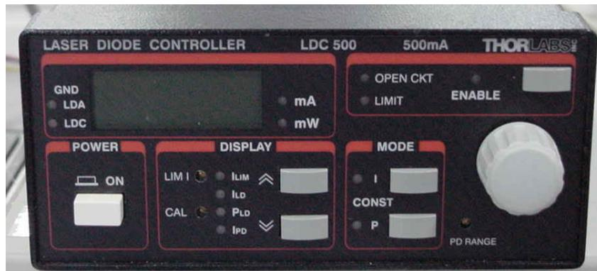
Figure 11. Thorlabs LDC 500 laser diode controller
