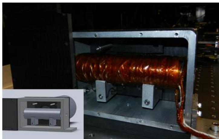
Figure 31 The heating tube used to house the gas cell. The tube is thermally isolated from the external housing to limit heat loss.
