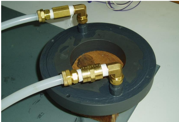
Figures 11 and 12: Photographs of the prototype coil. (left) The complete and sealed prototype coil with brass compression fit elbows connecting to polyethylene tubing. (right) The separating joint of the water and electrical supplies is shown.
