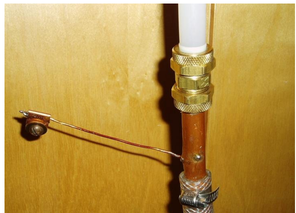
Figures 11 and 12: Photographs of the prototype coil. (left) The complete and sealed prototype coil with brass compression fit elbows connecting to polyethylene tubing. (right) The separating joint of the water and electrical supplies is shown.
