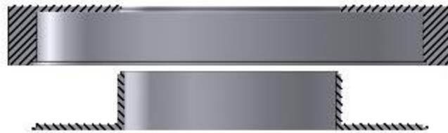
Figure 10: Supplemental IRONCAD drawing of the magnetic coil housing. The top piece ('hat') is fit over the coil and seals to the base piece, on which the coils are wound. Water and electrical connections are made on the bottom of the base piece.
