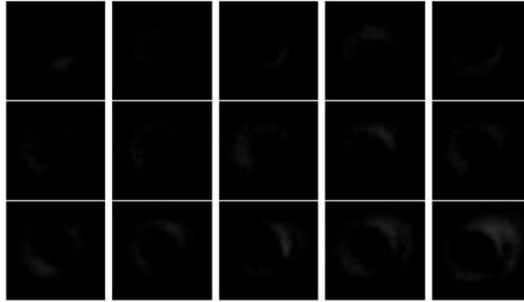
Figure 3.11: Subtracted images of beam at varying power. From left to right, top row to bottom row: 10W, 15W, 20-30W (at 1W increments), 35W, 40W.
