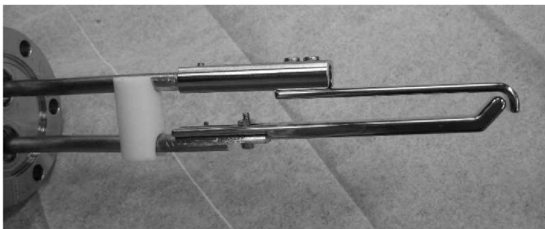
Figure 3.3: High DC voltage electrodes for use in the electric field induced Feshbach resonance experiment. The electrodes are attached to a 1.33” vacuum CF flange electrical feedthrough. Inserted into the vacuum chamber, the extended length will allow the electrodes to be placed physically close to the trapping region of the atomic gas. The spacing of the electrodes is approximately 1.3mm.
