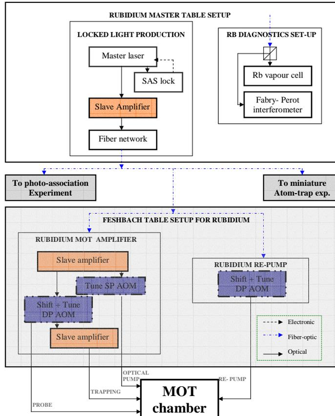
Figure 3.11: Flowchart summarizing the the optical procedure to create light to enable rubidium's laser cooling.
