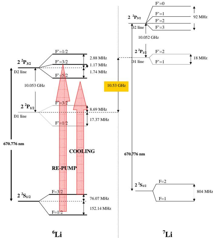
Figure 3.1: Schematic of lithium energy level diagram with the laser cooling and re-pump light shown for  ${}^6\text{Li}$ .  ${}^7\text{Li}$  energy levels are shown for comparison- and also since they overlap with some  ${}^6\text{Li}$  transitions. Refer to [47] for more accurate frequencies.
