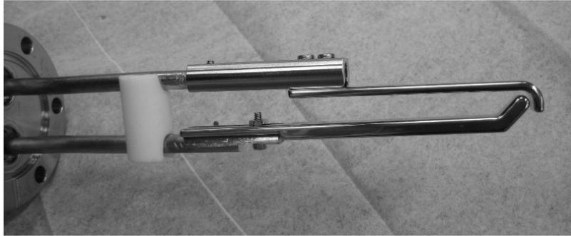
Figure 6.3: A picture of the high DC voltage electrodes attached to a 1.33” vacuum CF flange electrical feedthrough before being inserted in the vacuum chamber. The spacing between the electrodes at the curved end, where the cold atoms would be inserted is around 1.3 mm.
