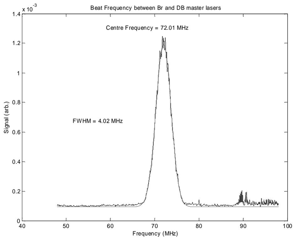
Figure A.2: Line-width of the master lasers as obtained by beating two locked master lasers. Assuming un-correlated errors, the line-width of our lasers is  $4.0 \text{ MHz}/\text{Sqrt}(2) = 2.8 \text{ MHz}$ .]
