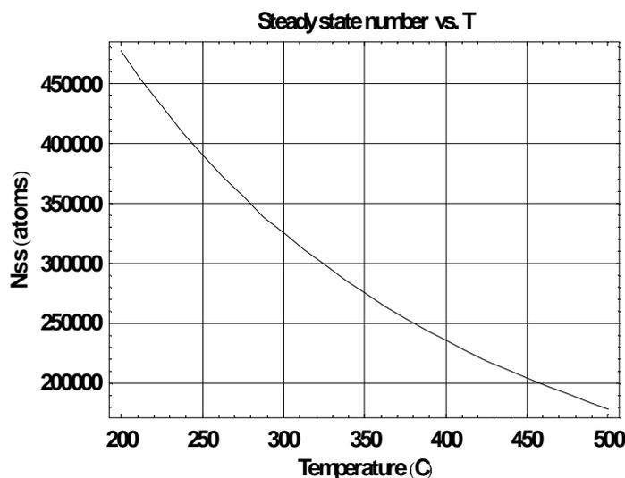
Figure 4.1: The calculated steady state number for trapped atoms in a lithium MOT as a function of temperature.
