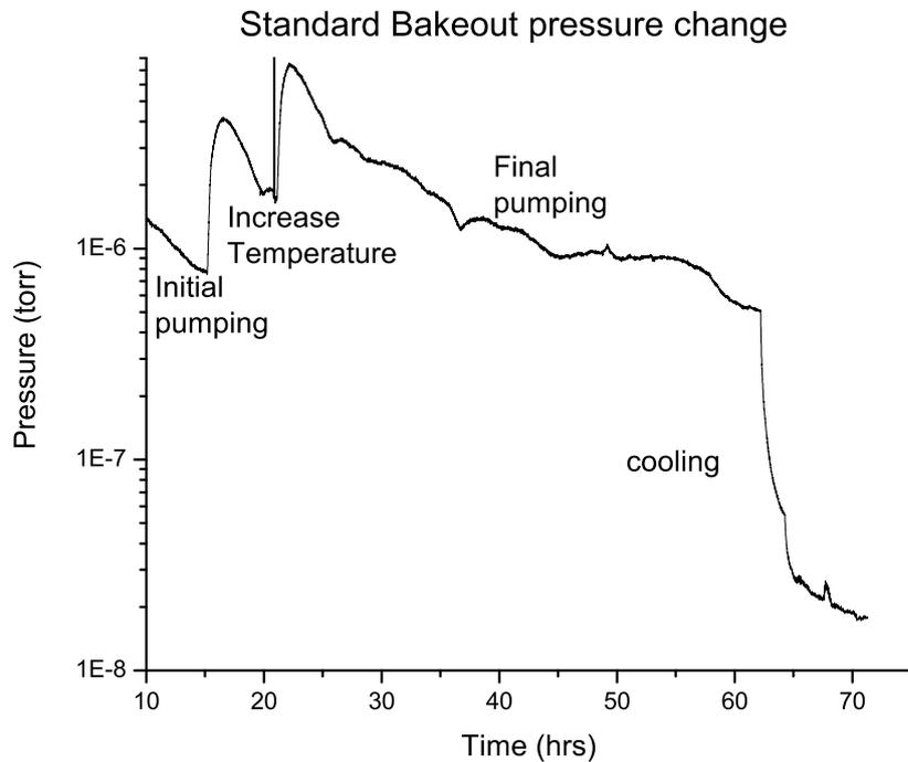
Figure 5.1: Figure illustrating part of the actual lab bakeout procedure. During an increase in temperature, the pressure increases considerably, but over a period of time, the impurities are pumped out, and the base pressure actually decreases considerably after cooling.
