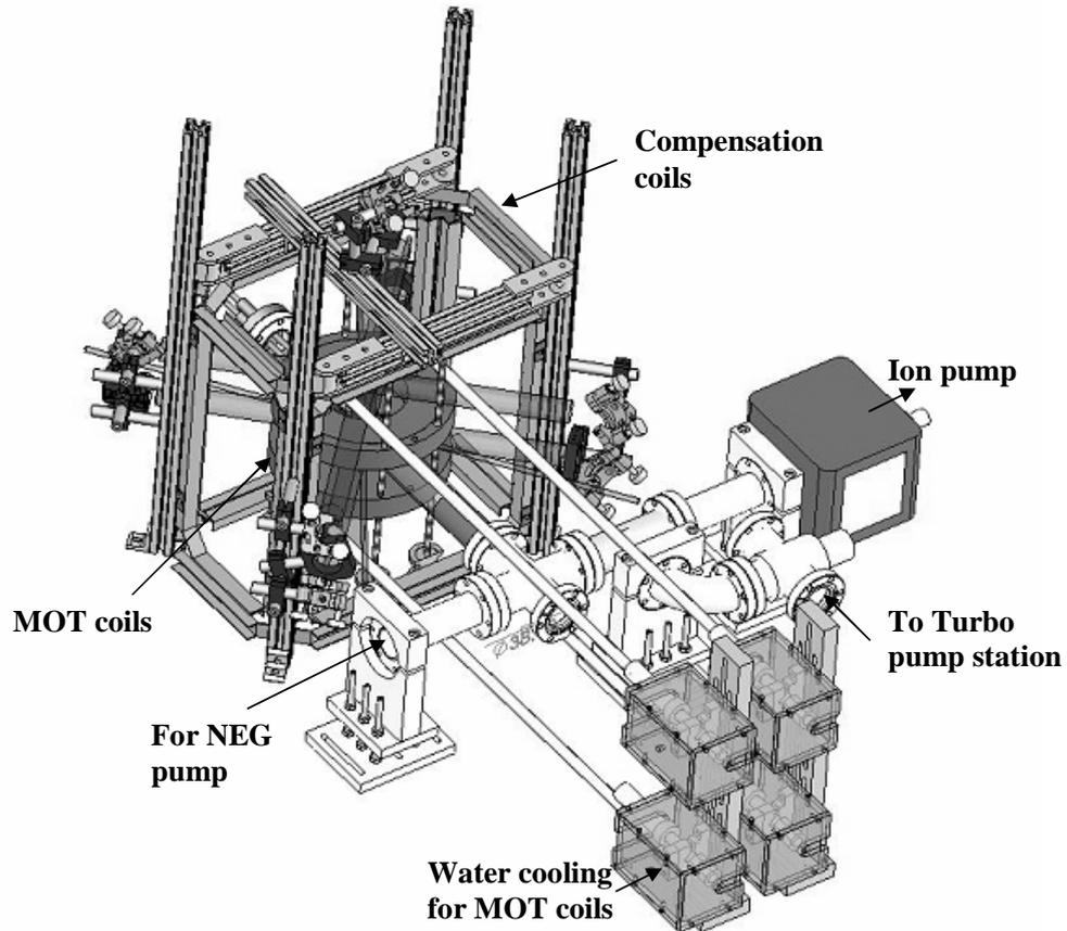
Figure 5.2: Solidworks drawing of the experimental arrangement for Feshbach experiment showing the vacuum system and placement of some optics.
