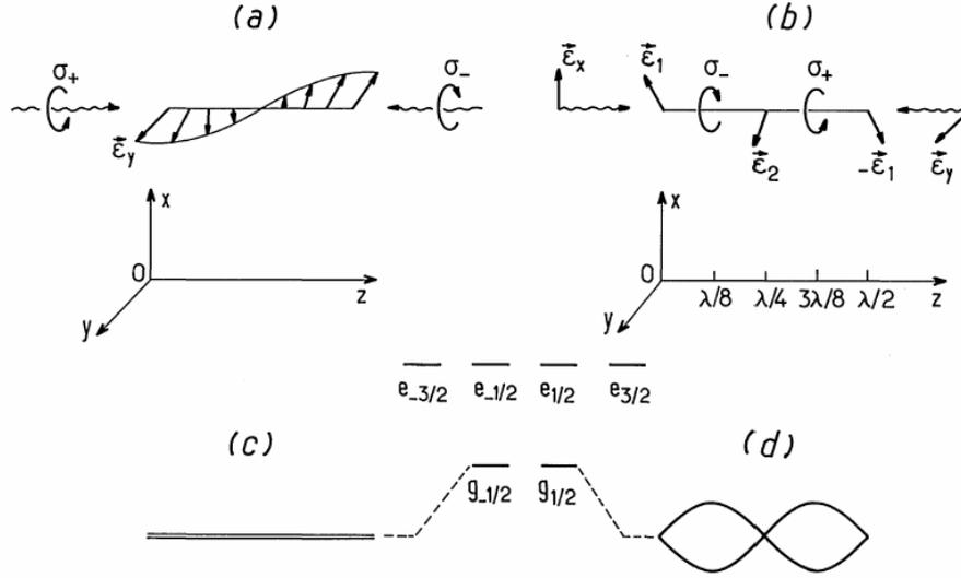
Figure 2.4: Schematic diagram showing the energy levels of a multi-level atom, with  $J=1$  being the lower state, in the presence of counter-propagating laser beams. Because the resultant polarization is different as a function of distance (as demonstrated in (a) for  $\sigma^+ - \sigma^-$  configuration and in (b) for 2 orthogonal linear polarizations), the energy levels are shifted appropriately (as demonstrated in (c) and (d)) leading to novel cooling mechanisms [figure from [23]].
