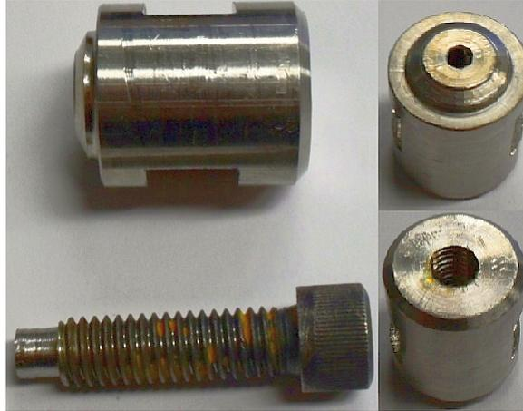
**Figure 2.3:** Different views of the stainless steel press designed to create a lithium rod by pushing chunks of lithium through a hole. The diameter of the hole matches the required diameter of the extruded lithium rod that is put into the oven. A slot for a 13/16 wrench was cut to prevent the press from rotating when the piston is screwed in.
