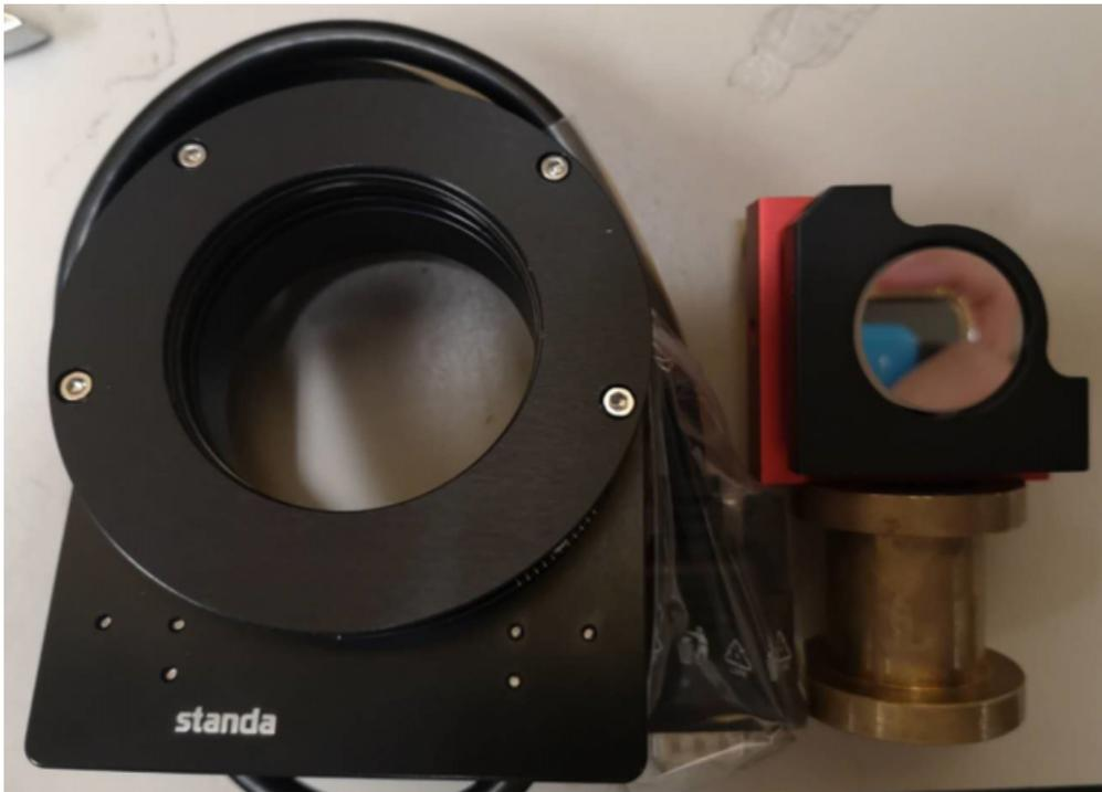
Figure A.1: A picture of the motorized iris. A one inch mirror is placed on the right to show a size comparison.
